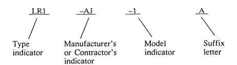
Type indicator. The type indicator of the designation shall consist of two parts: the letter symbol and the type number. The letter symbol shall be selected from Appendix E, Table E-II, indicating the type of propulsion device. The type number shall be assigned progressively by the DoDCP. The type number shall be arbitrary and shall not represent any characteristics of the propulsion device involved. These numbers shall begin with the lowest number not previously assigned to a propulsion device.
